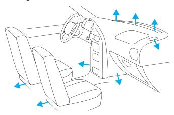
Rear seat heating is provided through the floor ducts located under the front seats. Airflow and temperature to the rear seating are regulated by the main climate control system.
